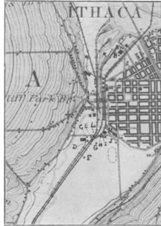
FIG. 1.—Section of the “Ithaca Sheet” (U. S. Geological Survey) to show the location of the artesian wells. A , B , salt wells, rock at 430 and 401 feet respectively; C , Strang Well, No. 1, 286 feet, struck rock at 260 feet; D , Millard Well, No. 2, 259 feet; E , Old Clinton St. Well, 280 feet; F , South Well, 232 feet; G , Strang Well, No. 2, 352 feet, struck rock at 342 feet; H , Trapp Well, 332 feet; I , Holmes Well, 291 feet; J , Millard Well, No. 1, 303 feet; K , several wells, close together, as follows: Illston Well, 286 feet; Strang Well, No. 3, 280 feet; Strang Well, No. 4, 279.9 feet; Strang Well, No. 5, 276 feet; and Strang Well, No. 6, 295 feet; L , Millard Well, No. 3, 303 feet.
